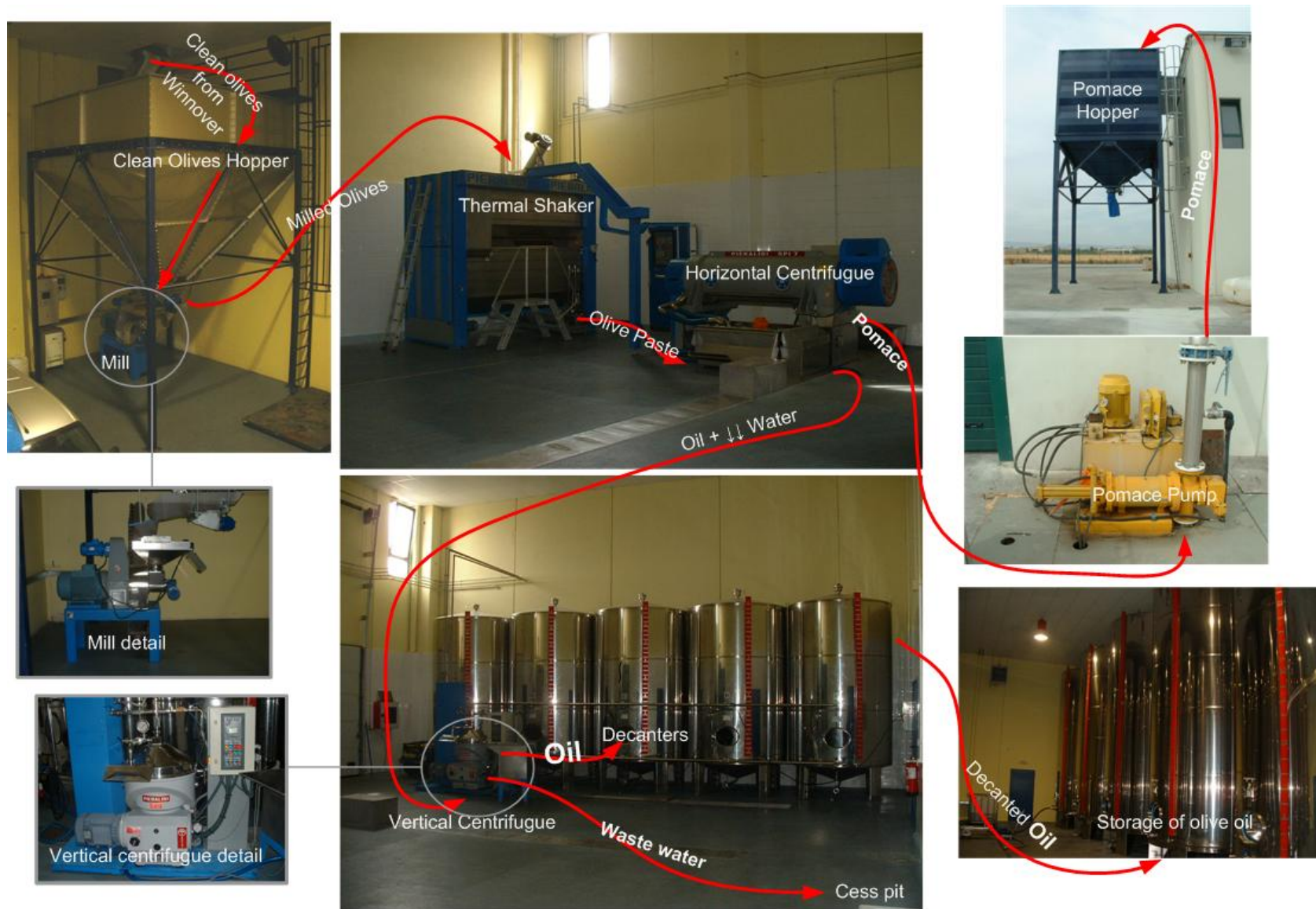
Figure 42. Obtaining and storage of extra virgin olive oil in Almazara del Ebro
